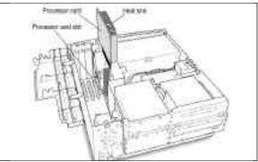
Installing the MACh Speed G3
